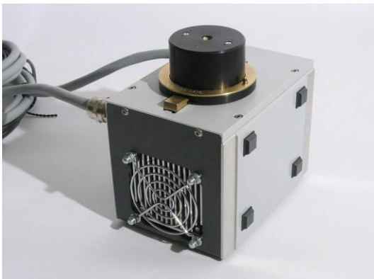
Fig. 1: Test fixture with Peltier based active cooling, FEM simulation of the heat sink
